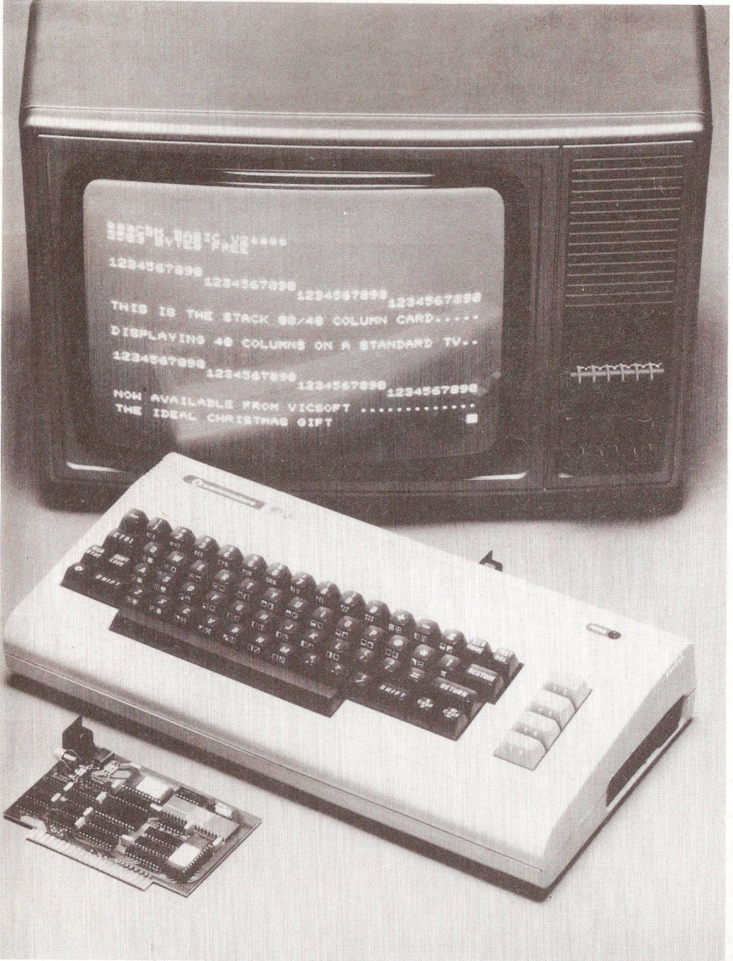
The stack 40/80 column card for the Commodore VIC-20
